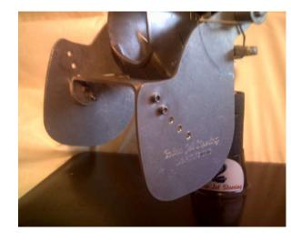
This picture shows the fins staggered. While in the down all the time mode. This is an option for twin engine boats where the operator wants to reduce the amount of high speed assistance without eliminating it all together. Setting the outer fin up on both nozzles will accomplish this. The higher you set the outer fin, the less exposure and therefore the less effect it will have at planning speeds. On single engine boats the fins
