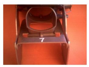
The actuator attaches the two fins together to stabilize them to resist flexing, plus it allows for separate fin adjustment when being used in the all time assist mode.
