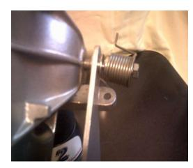
(One more picture of the right side fin being installed to show the spring is not loaded yet. Note this picture shows a metal reverse gate, these units are compatible with the metal or plastic reverse gates.)
