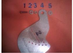
This picture shows the proper sequence of parts for the left fin installation using the new plastic reverse hood bolt, flat washer, bushing, fin, second flat washer and the original factory bushing for the
