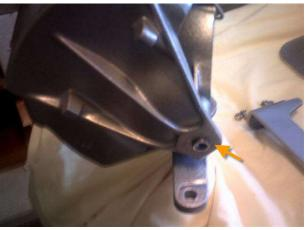
This picture shows the correct parts and correct sequence for placing those parts onto the long hex bolt listed as **#1**, next is the large thin flat washer listed as **#2**, place that washer on the bolt, next
