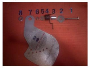
fin listed as #7 with the writing facing out and the large part down. Next you need to place the second washer listed as #8 on the bolt.
