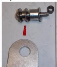
The 8mm button cap bolt has a flat washer then the .218 spacer whee the fin mounts then another flat washer and the 9/16 aluminum spacer and another flat washer, the small round piece at the end is the original reverse bucket standoff that must also be reinstalled just like on the other side so that the reverse can operate properly.
