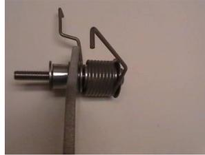
the fin 2.18 spacer; this is where the fin mounts in the sequence.
