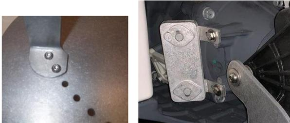
We now need to reposition the anodes located on the left side of each pump. We have provided you with repositioning brackets bolts and nuts to accomplish this.
