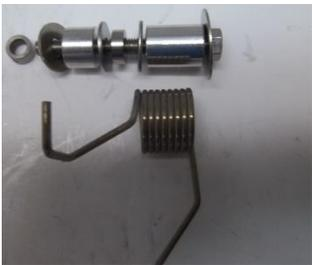
These are the parts first the long 8 mm hex bolt then the large thin washer next the 1-inch long aluminum spacer for the spring to sit on next the spring with the longer arm on closest to the bolt head. Then a washer and then the .218 fin spacer where the fin will be placed: see top picture with arrow.
