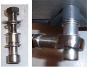
attached to the nozzle with tie rod, spacers & washers to lower the rod
