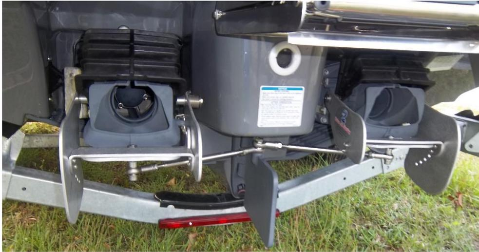
The new SUPER ULTIMATE A K-19 DELUXE SYSTEM is spring loaded, adjustable & selectable. You may choose to keep the fins in the water at a variety of different influence levels –OR- you may set the fins to rise up on plane and deploy for idle speeds and docking when off plane.
