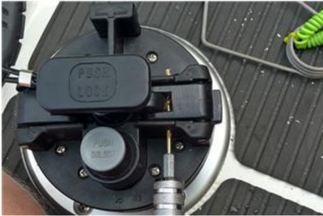
#4 Drilling the hole Close up of where to Drill (as stated in # 4)
