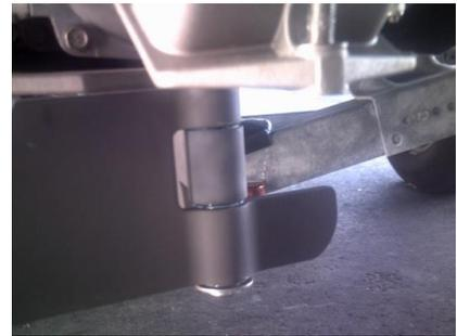
**Step #3.** Move the rudder sideways toward the front of the nozzle to allow for the **VIPER** to slide over the castings on the nozzle and into position on the bottom edge of the nozzle. As shown in the pictures.
