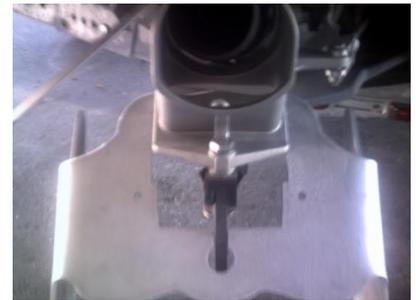
**Step #4,** rotate the rudder back to its original position now or after your installation is complete your choice, remember to place thread locking compound on the retainer bolt when reinstalling it.
