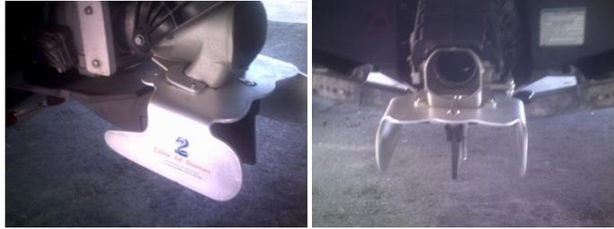
**Step #1.** Simply place the controls in forward to open the reverse bucket allowing you easy access to the back of the nozzle.
