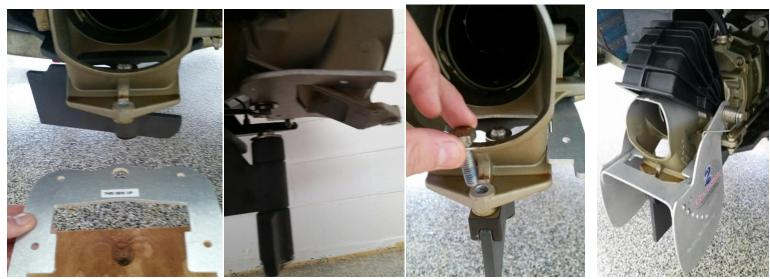
Once the side force stabilizer is installed properly you can reinstall the rudder bolt and retainer, be sure to use thread locking compound on the bolt. Now you can proceed to finish the installation of the fins etc. per the regular instructions.
