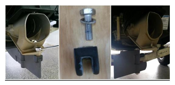
First remove the bolt and retainer that attaches the end of the nozzle to the rudder.
